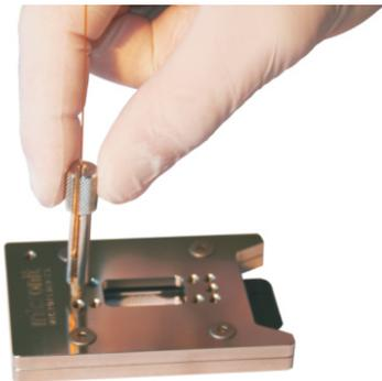
Figure 5.1. Extender tool, for 1/4 or 1/3 round additional tightening
