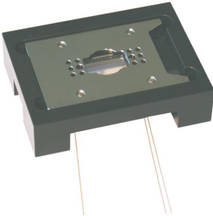
Figure 3.1. Chip holder upside down in the chip holder frame
