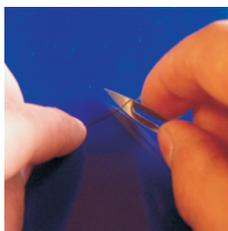
Figure 2.5. Cutting the capillary
