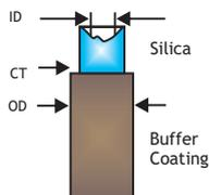
Figure 2.4. Fused silica with a polyimide coating
