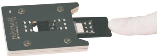
Figure 2.2. Slide the chip into the chip holder
