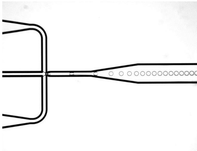
Figure 5: Droplet can be oil-in-water or water-in-oil.
