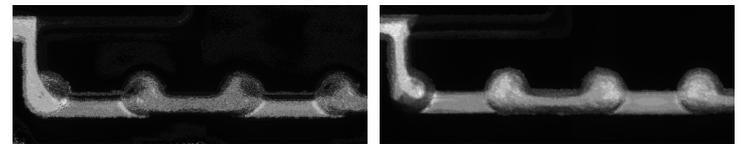
The images show the first few elements of the swirl mixer at Re = 0.25 (left) and Re = 250 (right). The effect of inertia is clearly evident with the two bands of fluid passing unaltered through the mixer at low Re number compared to a significant reduction in mixing length due to the swirl at high Re number. The computations suggest that the swirl mixer operating in the inertial regime will be the most efficient mixing solution and the evidence from the flow visualisation supports this.
